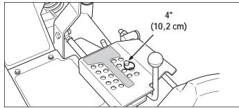
Figure 40. Deck Height Pin Position
